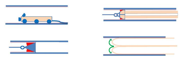
The slurry of cleaning water discharged during the cleaning operations and the material that has been brushed and brought outside the pipe (*due to rubbing against the internal surface of the AC pipes that, after a long time of service, could be deteriorated*) can contain a high concentration of asbestos fibers that had to be assessed and appropriately disposed of.
