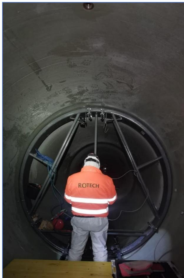
Figure 8. Execution of leak test on single joint
