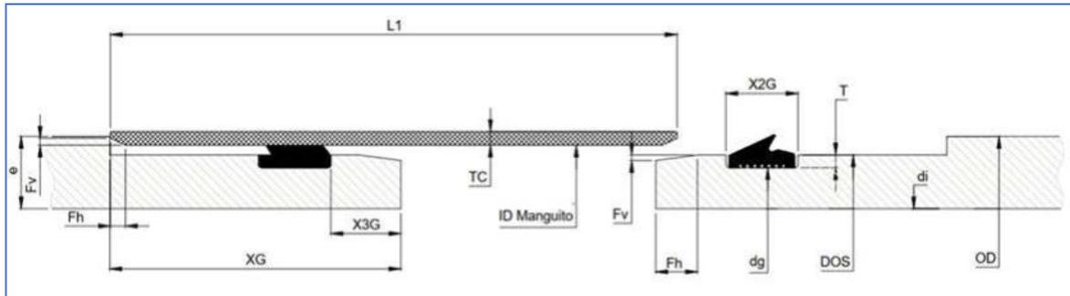
Figure 3. Pipe-sleeve coupling system detail.
