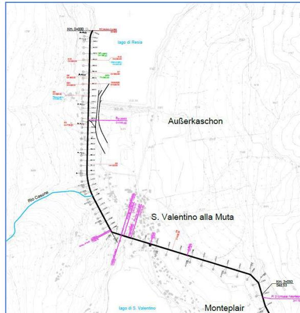
Figure 1. Plan layout of the diversion tunnel
