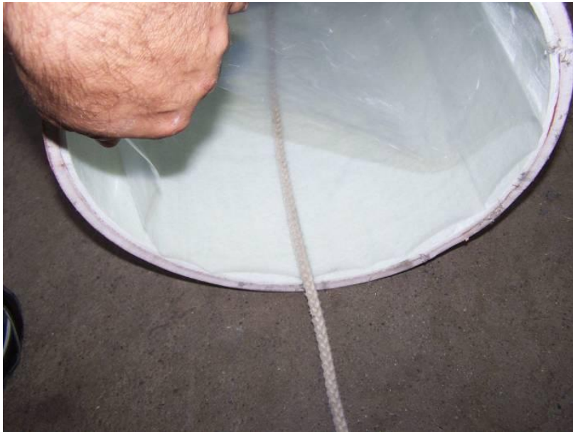
Figure 10: Release of inner film after curing
