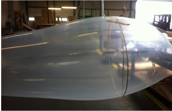
Figure 4: Expansion test of inner film
